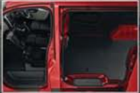
A 1.0M wide sliding door is available for one or both sides.
